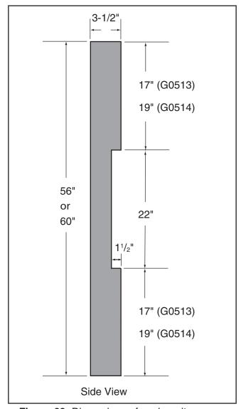
Figure 62. Dimensions of coplanarity gauge.
